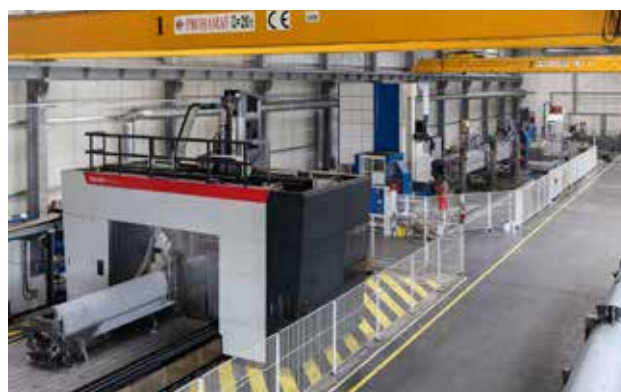
Telemond | Automatic welding line for telescopic booms
